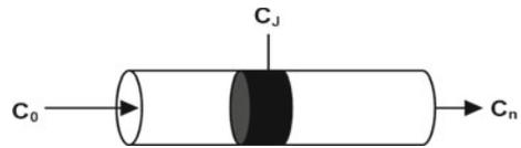
The material balance relation for the particles in the fluid stream, flowing through an element of porous medium can be represented by the following expression:
