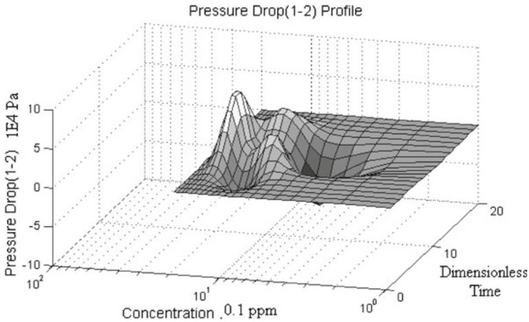
**Fig. 13** Pressure Drop as a function of dimensionless time and concentration
