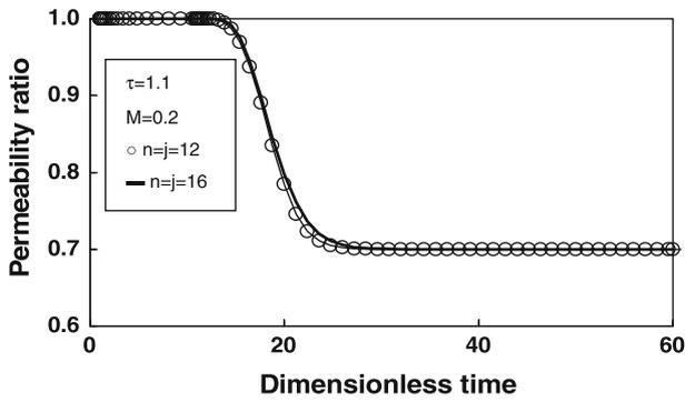
**Fig. 11** Permeability ratio as a function of dimensionless time with considering time lag and the number of elements
