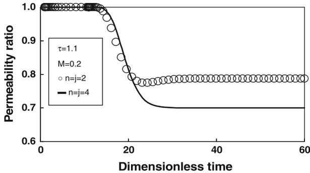
**Fig. 8** Permeability ratio as a function of dimensionless time with considering time lag and the number of elements
