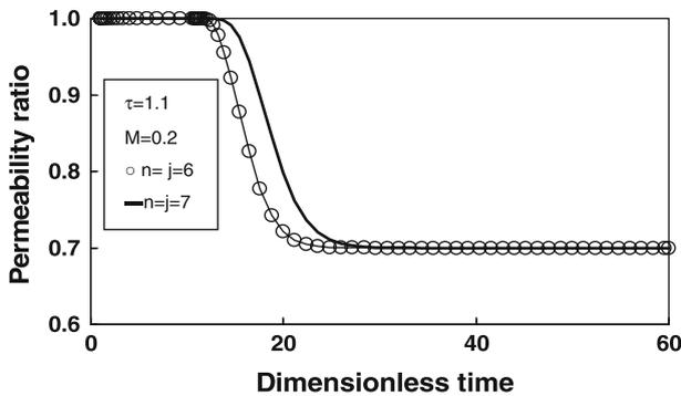
**Fig. 9** Permeability ratio as a function of dimensionless time with considering time lag and the number of elements
