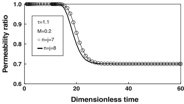
**Fig. 10** Permeability ratio as a function of dimensionless time with considering time lag and the number of elements
