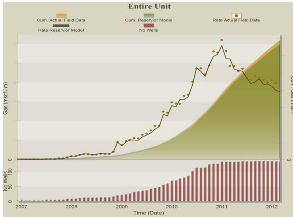
Figure 6. History matching result for entire field by using the maximum possible combination of Parameters
