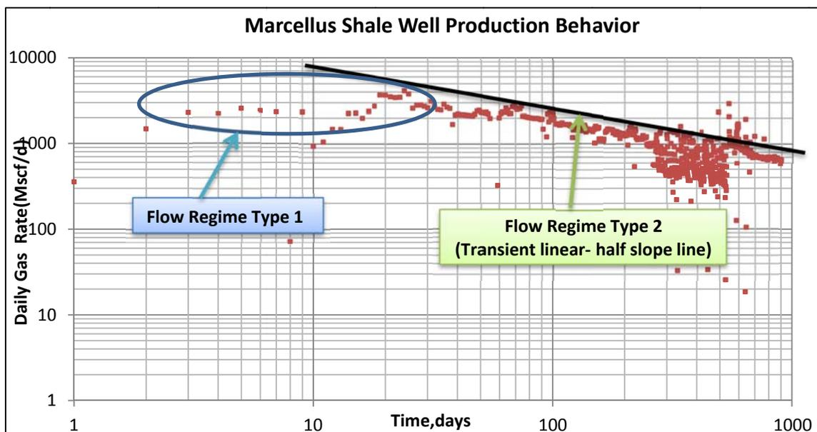
Figure 4. Log-log plot of production rate as a function of time for one of 135 wells
