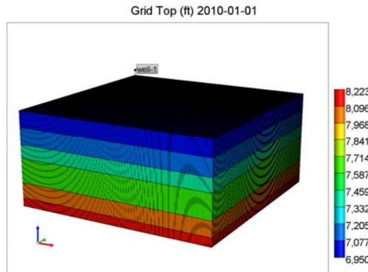
**Figure 4. Dynamic model for the Mattoon CO<sub>2</sub> injection site**
